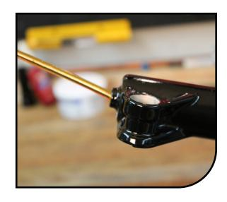
Using an 8mm Allen wrench tighten the rebound damper rod and air spring assembly to 35–40in lbs [3.95–4.5 Nm] by turning them **counter-clockwise**. Do not overtighten, doing so can damage the end of the rods.
