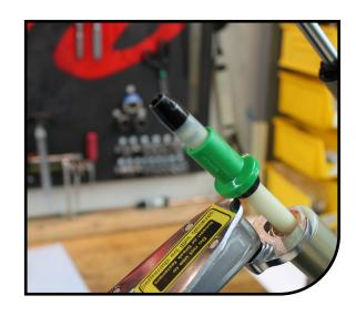
Attach a shock pump and inflate air leg to 30-50PSI. This will aid in installing the casting later.
