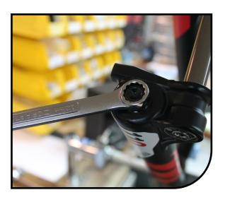
Remove casting from fork. It is recommended this be done over a drain pan as the lower casting contains semi-bath oil. Allow oil in casting to drain out before continuing to next step.
