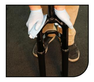
Pour additional 5wt fork oil into the damper leg until the oil height (space from the top of the damper leg to the top of the oil) is set at the proper level. See following page for the correct oil height depending on compression damper type and fork travel. An oil height setting tool used for motorcycle forks similar to the one pictured makes this job easier.
