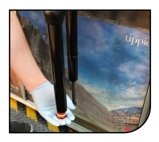
Take new Air Piston out of bag and liberally grease the piston quad seal and outer surface with Slickoleum™ grease.
