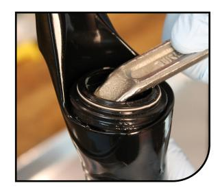
Remove old foam wiper rings. Apply semi-bath fluid to the new foam wiper rings and install into fork casting.
