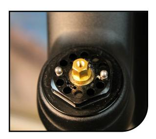
Unthread ABS+ compression damper assembly from the stanchion using a 24mm socket and ratchet. If the fork has the Kwik Toggle compression damper you will need to use the Mattoc Cassette Tool and 1" wrench or socket to remove the damper.
