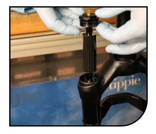
If installing an ABS+ damper use a 24mm socket and torque wrench, tighten the damper to 60–80 in lbs [6.8–9.0 NM]. If installing a Kwik Toggle damper use a 1" socket or crow's foot, the Mattoc Cassette tool and a torque wrench to tighten down the damper to the same torque specification.
