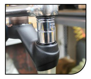
Invert the fork and use a 22mm box end wrench to unthread the air spring assembly from the stanchion.
