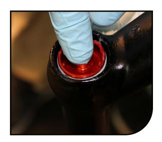
Add 8cc's of Slickoleum™ grease to the top of the air piston.
