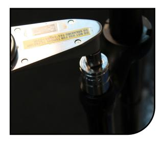
Install air spring assembly into stanchion. Using a 22mm crow's foot, tighten assembly end cap to 80-100 in lbs [9.0-11.3 NM].
