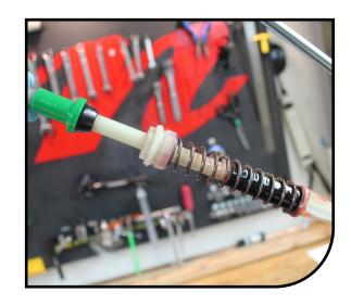
Using a long dowel rod or similar tool push the air piston down the stanchion and out of the bottom. Be careful to not scratch the inner surface of the stanchion. Once the piston is removed clean the inside of the stanchion with isopropyl alcohol and a lint free towel. Inspect the inside and outside of the stanchion for scratches or other damage.
