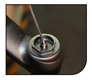
Remove air cap using a 20mm socket.
