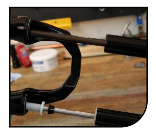
Insert 15cc's (15ml) of semi-bath into each casting leg. Once the semi-bath is in the legs slide the casting the rest of the way onto the stanchion assembly.
