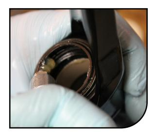
Fill the air chamber with a small amount of air (20-30PSI). This will extend the air spring assembly and make casting installation easier.
